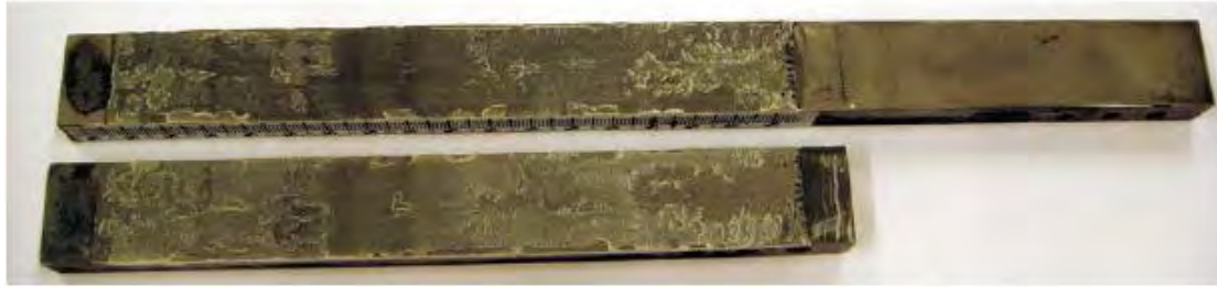
Figure 17 Example of failure surfaces obtained with the SLB test.
