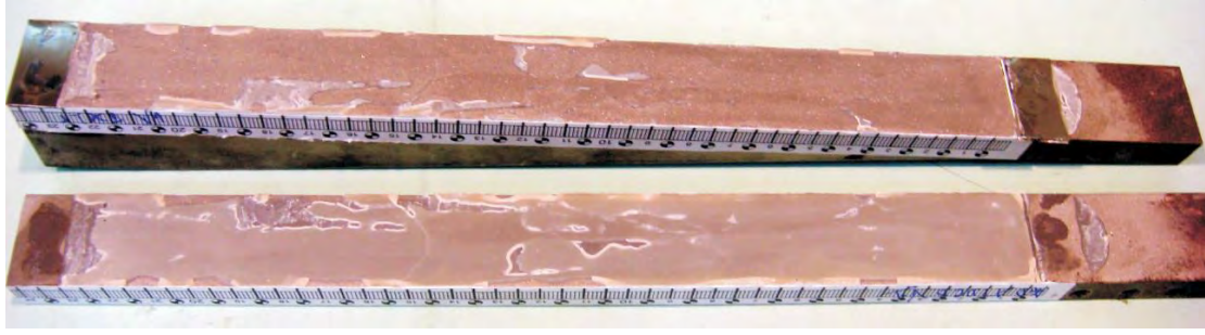
Figure 23 Example of failure surfaces obtained with the ATDCB test.
