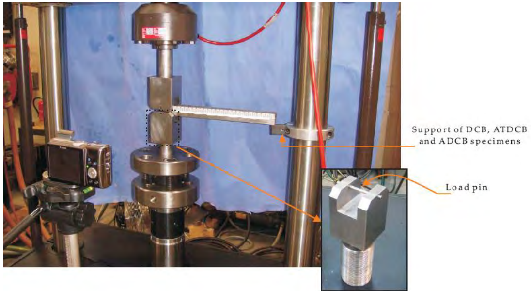
Figure 8 Experimental set-up of the tests in opening mode (DCB, ADCB and ATDCB).
