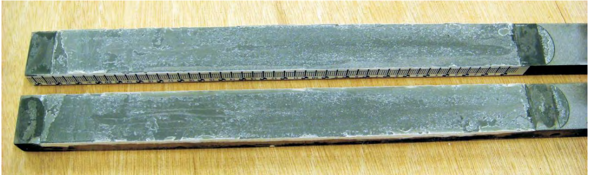
Figure 11 Example of failure surfaces obtained with the DCB test.
